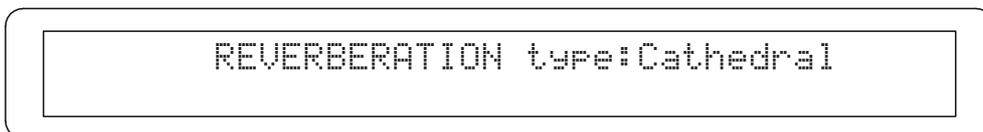
Use the encoder to select the type of reverb and press [EXIT] to save the selection and return to the SET-UP menu.
