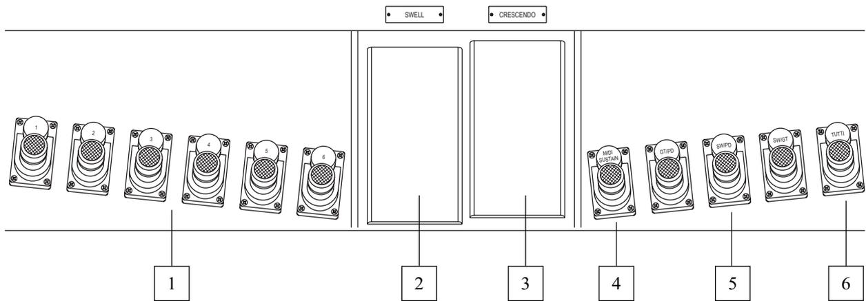
1. **General memory pistons:** these pistons can be used to recall the organ general memories.
