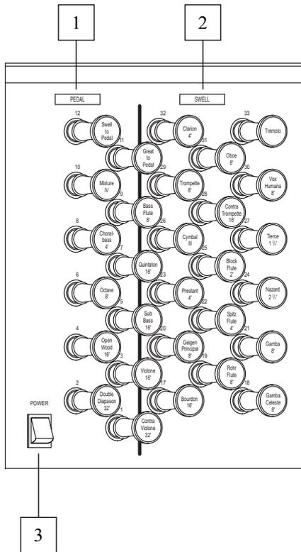
1. **[PEDAL] drawstops:** this section contains the first ten voices of the pedal board and couplers:
