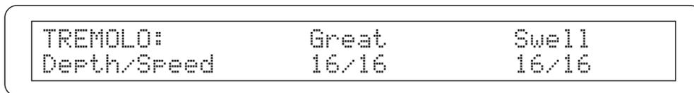
which shows the two manuals and, on the bottom line, the **Depth** (modulation depth) and **Speed** (modulation speed).
