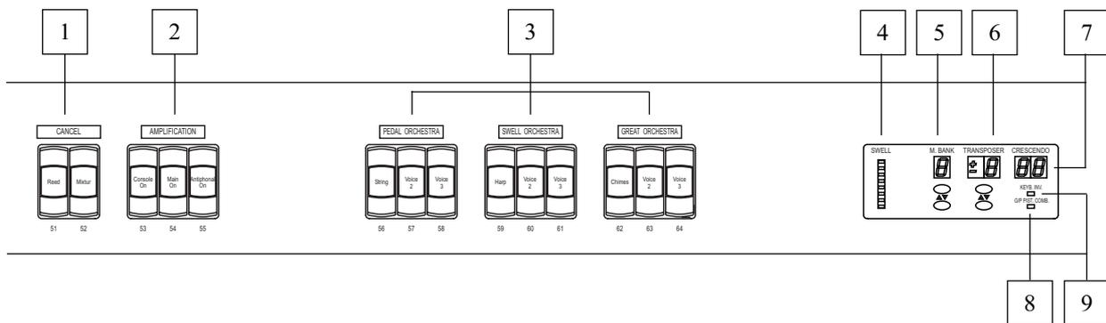
1. **CANCEL section:** these controls can be used to exclude all of the reeds (**[REEDS]**) and/or mixtures (**[MIXTURE]**).
