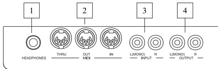
1. **[HEADPHONES] socket:** Jack socket to which a headphone set can be connected. With headphones connected, the organ's internal amplification is cut off.
