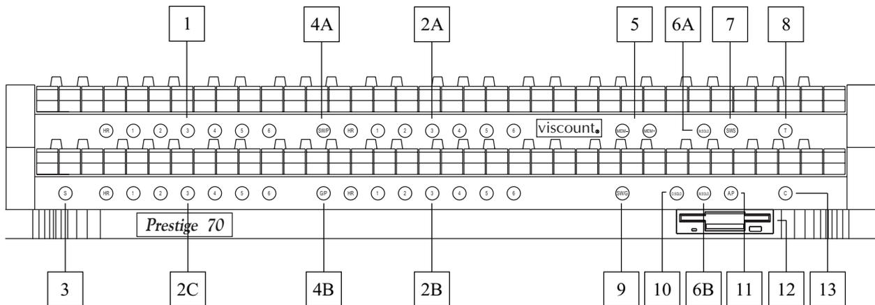
1. **General memories:** this section contains the instrument's general memories. The [MEM+] button (point 5) can also be used to select the individual memories in ascending order and [MEM-] to recall them in descending order.
